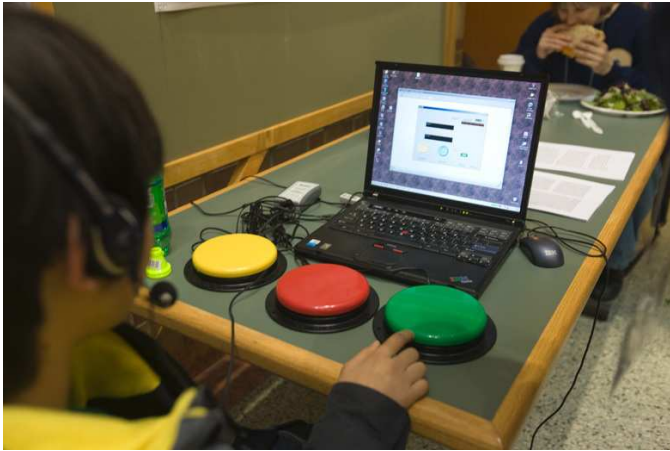
Fig. 1. Hardware setup for the Speech Recognition Game . Red, green and yellow external buttons were used to accept all non-speech user inputs. A green bar, displayed on the computer monitor, rose with each recognized word, to peak at ten correct recognitions.
