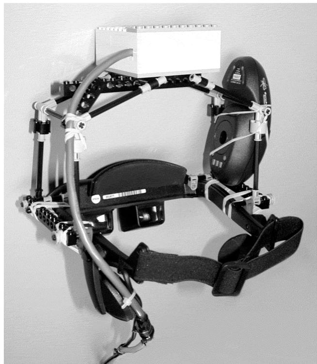
**Figure 1.** The head-mounted display. The white box on top contains the compass module. The dark ovoid on the side is the GyroMouse, which has a wireless connection to the backpack. The display units do not obstruct peripheral vision, so it is safe to walk (slowly) while wearing the HMD.
